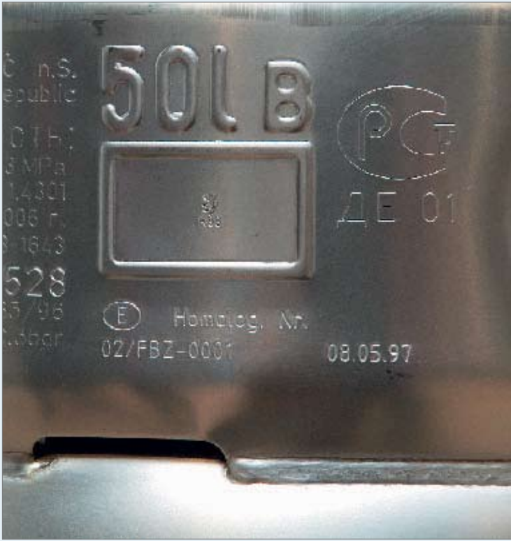
Figure 4. Weld connecting the top ring to the drum of a beer barrel. Welds are brushed before acid cleaning in HF and HNO 3 to remove discoloring and graphite particles.
