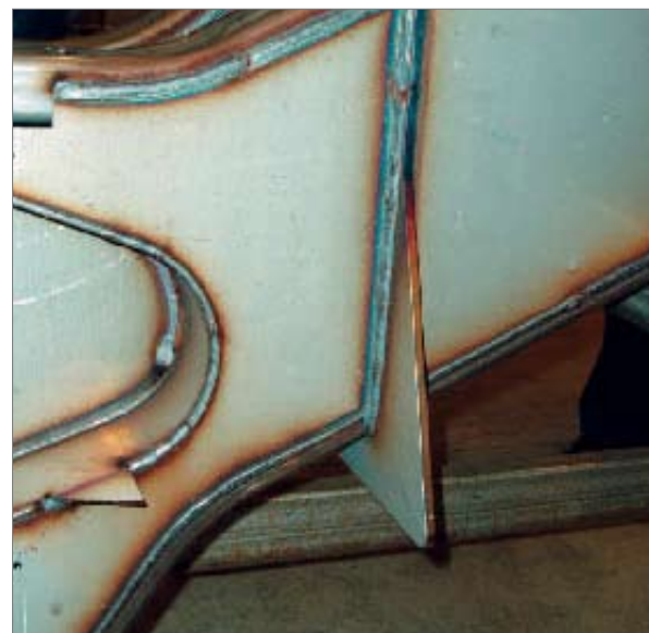
Figure 2. Examples of welded joints. The complete application included overlap joints, corner joints, fillet welds and butt welds.
