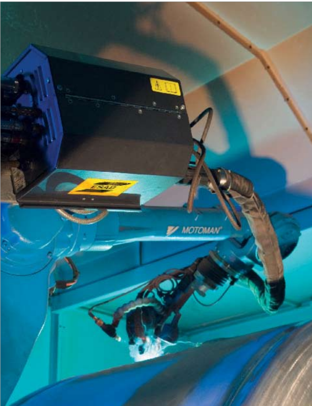
Figure 4. The tack welding of the backing bar as such, already shows the kind of precision applied in the welding of this advanced medical equipment.
