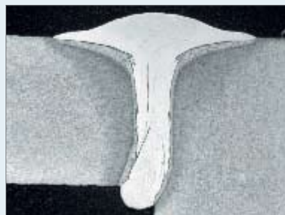
Figure 5. Corner joint. Note that the "laserfinger" is actually guided out of the joint into the root. This results from an intentionally induced root gap, so that the light is partially reflected by the joint faces in the root.
