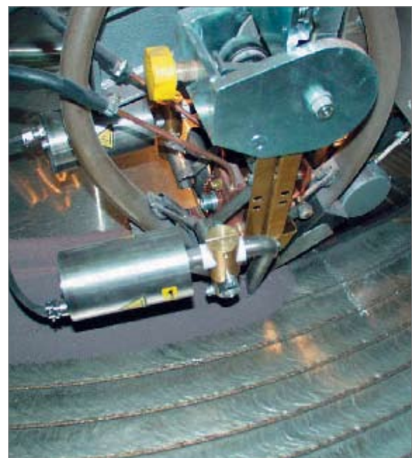
Figure 1. Strip cladding of vessel head by submerged arc welding (SAW).
