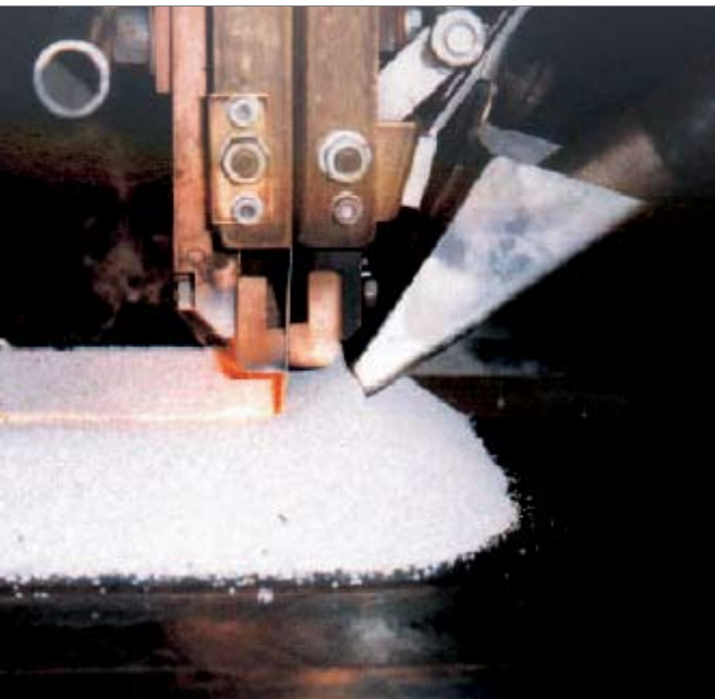
Figure 5a and b. Electroslag strip cladding of a refinery reactor at Sices.
