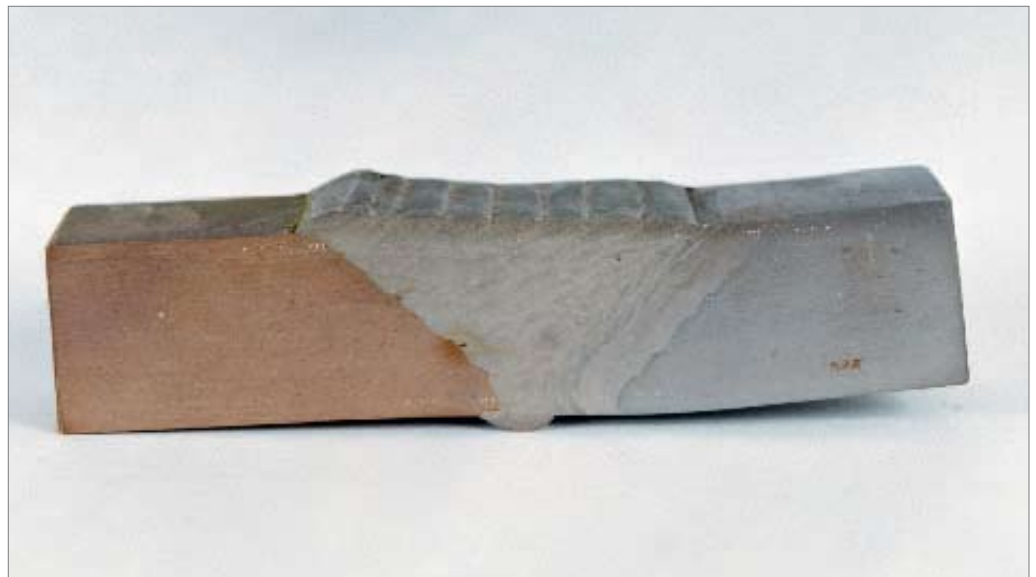
Figure 3 . Macro of a PQR sample of an 'exotic' joint in a desalination installation. 22 mm thick Cu/Ni 90/10 (left) connected to 20 mm thick S 31803 duplex stainless steel (right), welded with manual TIG with automatic wire feeding. The duplex side is first buffered with two layers of OK Autrod 19.92 (ERNi-1) followed by two layers of OK Autrod 19.93 (ERNiCu-7). Subsequently, the two sides are joined with OK Autrod 19.49 (ERCuNi). One layer, with the (acceptable) pore, is welded with MIG, just to get the process approved.
