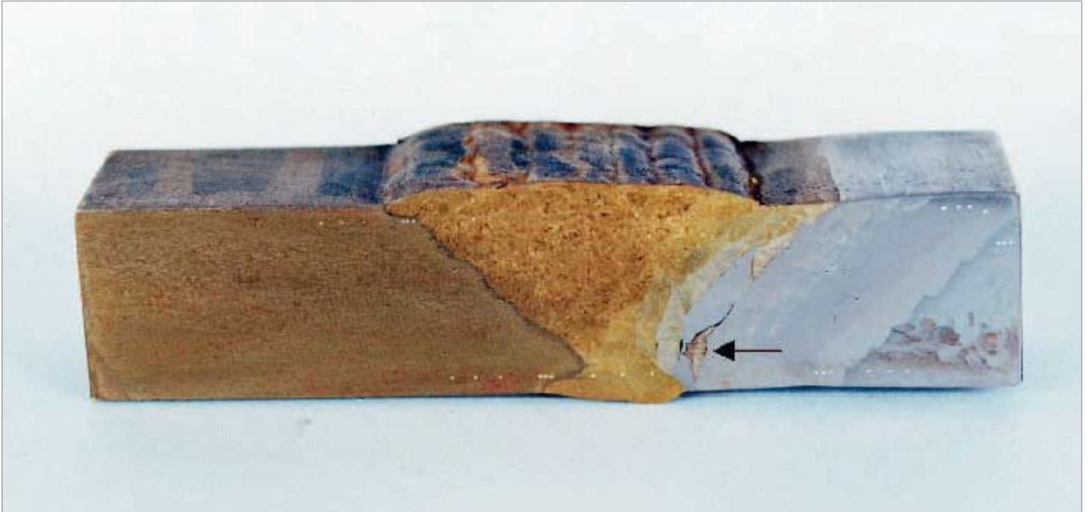
Figure 4. Another example of an exotic joint. Macro of a PQR. 22mm thick CuAl (UNS C61400) connected to 20 mm duplex stainless steel, welded with semi-automatic TIG with automatic wire feeding. The duplex material (right) is buffered with two layers of OK Autrod 19.92 (ERNi-1), two layers of OK Autrod 19.93 (ERNiCu-7) and finally with four layers OK Autrod 19.49 (ERCuNi-7). Subsequently, the two sides are joined with OK Autrod 19.44 (ERCuAl-A2). One layer is welded with MIG, just to get the process approved. On the duplex side, all buffering layers have been dye-penetrant tested. The first layer of OK Autrod 19.44 (ER CuNi) showed minor indications of cracking. These areas were ground out and repaired with OK Autrod 19.49 before continuing with OK Autrod 19.44. The arrow shows the repaired area on the macro photo.
