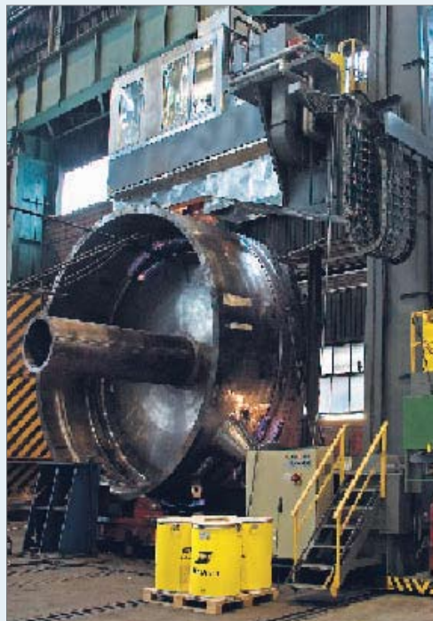
Figure 7. Narrow-gap welding of a circumferential joint. Welding wire is fed from 280kg drums to avoid costly downtime for spool exchange.
