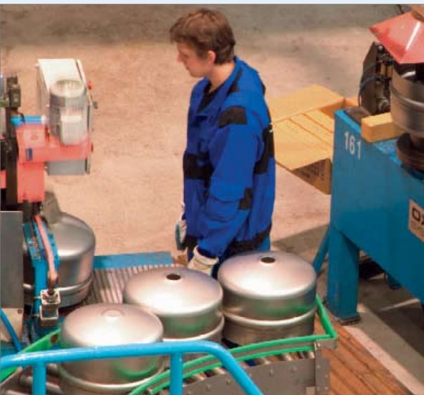
Figure 2. Top drum section. The orifice for the outlet valve is punched through within the designated reinforced area.
