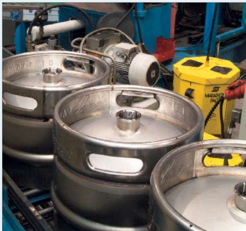
Figure 3. One step further in the process. The outlet valve and the top ring have been welded onto the top half of the drum using automated MIG welding stations. OK Autrod 308LSi stainless welding wire is fed from the Mini Marathon Pac to the various welding stations and pulse welded under Ar/4% CO 2 shielding gas.
