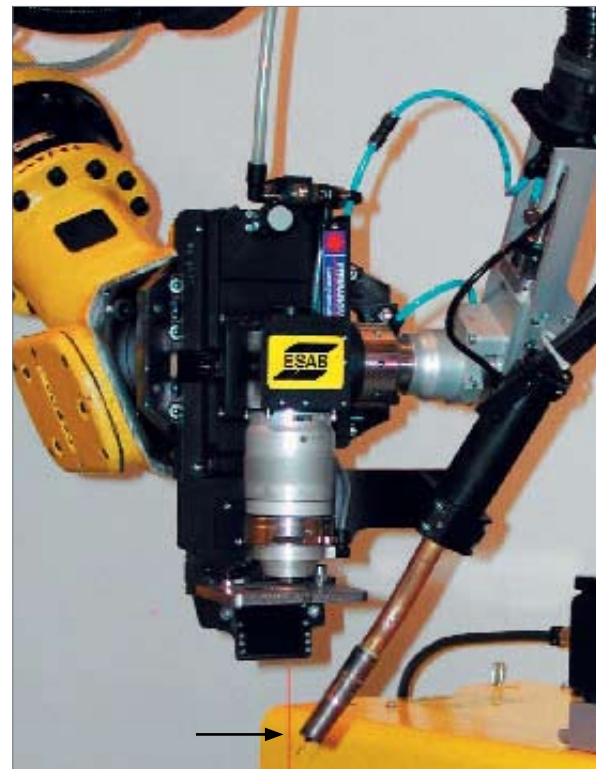
Figure 1. Laser-hybrid welding head. The arrow shows the point where the laser light and the MIG arc join into the hybrid process.
