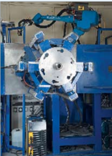
Figure 3. Motoman robot equipped with the Aristo™ robot package and internal clamp/manipulator.
