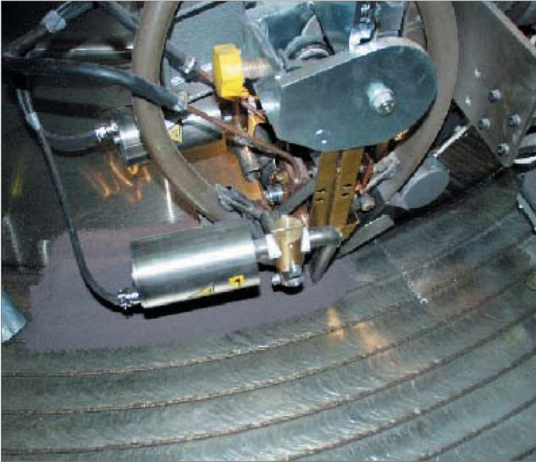
Figure 8. SAW strip cladding of a heat exchanger component.
