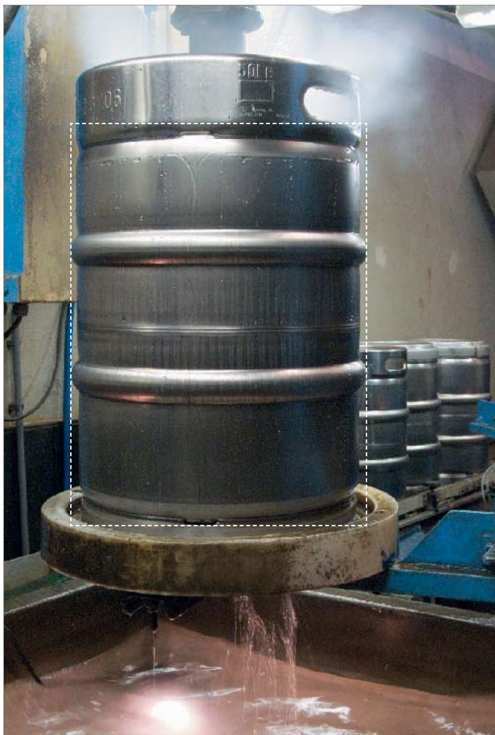
Figure 1. Finished beer barrel during pressure testing at 35 Bar. The top ring with hand grips and the drum (dotted area) are fully visible. The base ring is partially covered by the clamp from the testing equipment. The central circumferential joint is TIG-welded without consumables. The top and base rings are MIG-welded to the drum.
