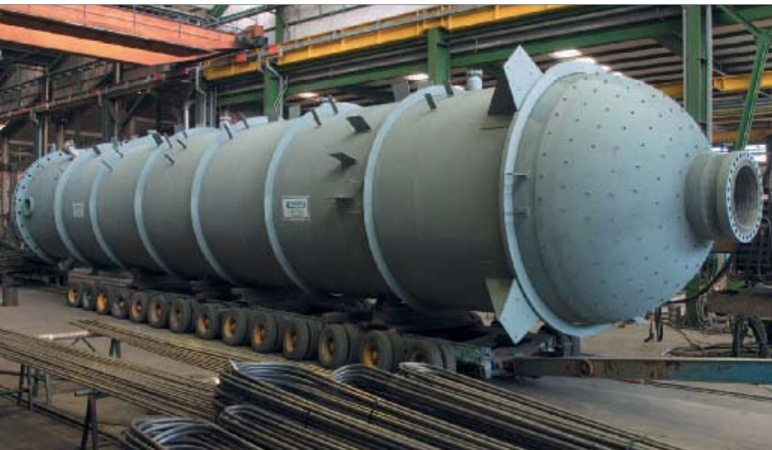
Figure 2. – Reactor for refinery - desulphurization plant at sices.
