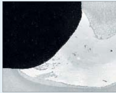
Figure 4. Cross section of a fillet weld. Note the brilliant transition to the parent material.
